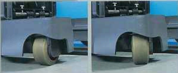
Higher Maneuverability with multi-angled wheels
